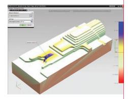
Feature recognition. The power of feature recognition has expanded greatly, with the recognition of more features in more scenarios than ever. Multi-stepped holes, including chamfers and rounds are recognized. Additional flats, slots and pockets are recognized also.
