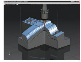
and Cross curves can be determined automatically or fine-tuned by the user to achieve the smoothest, finest finish possible with improved tool life. Streamline operations can be applied to 3-axis or 5-axis cutting scenarios.
